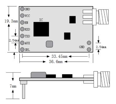
Figure 34: Mechanical Dimensions
