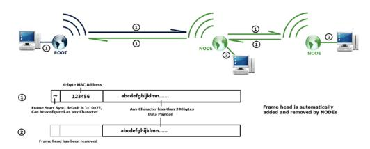
Figure 12: Frame Structure of Half Transparent Transmission
