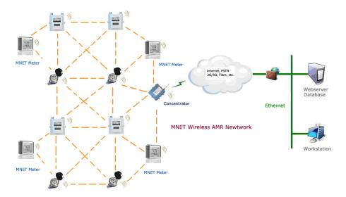
Figure 28: Wireless AMR Network Based on MNET III
