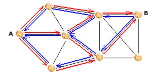
Figure 5: MNET III Multi-path Routing
