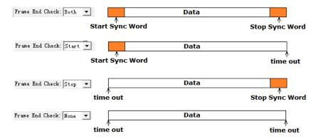
Figure 17: Synchronization Words in ASCII Frame Mode.
