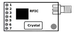
Figure 1: DRF1110N Pin Layout
