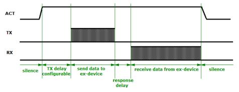
Figure 10: Two-way Communication of ACT, TX and RX Pins
