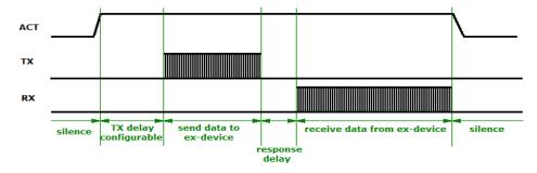
Figure 16: Time Sequence for TX Delay
