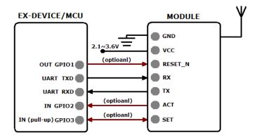
Figure 8: DRF1110N Connection Diagram
