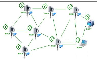
Figure 26: Wireless Sensor Network
