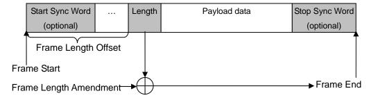
Figure 19: Variable Frame Length in Binary Mode
